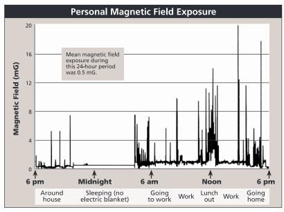
In the above example, the magnetic field was measured every 1.5 seconds over a period of 24 hours. For this person, exposure at home was very low. The occasional spikes (short exposure to high fields) occurred when the person drove or walked under power lines or over underground power lines or was close to appliances in the home or office.
