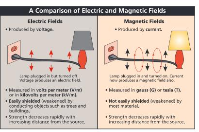
An appliance that is plugged in and therefore connected to a source of electricity has an electric field even when the appliance is turned off. To produce a magnetic field, the appliance must be plugged in and turned on so that the current is flowing.
