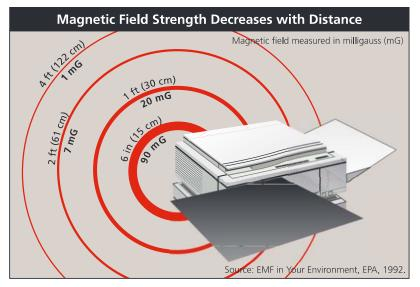
You cannot see a magnetic field, but this illustration represents how the strength of the magnetic field can diminish just 1-2 feet (30-61 centimeters) from the source. This magnetic field is a 60-Hz power-frequency field.
