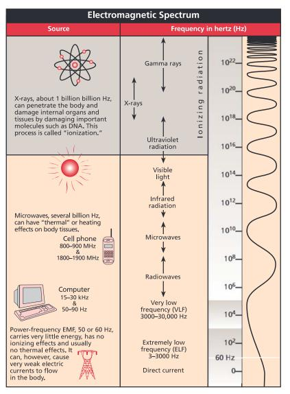
The wavy line at the right illustrates the concept that the higher the frequency, the more rapidly the field varies. The fields do not vary at 0 Hz (direct current) and vary trillions of times per second near the top of the spectrum. Note that  $10^4$  means  $10 \times 10 \times 10 \times 10$  or 10,000 Hz. 1 kilohertz (kHz) = 1,000 Hz. 1 megahertz (MHz) = 1,000,000 Hz.
